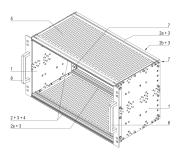
Subrack for Railway applications, conform to EN50155 standard, shielded versions.
