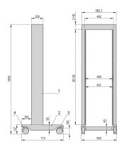
Open frame rack with 200 kg load capacity and recommended chassis depth of upto 400 mm, ideally for general electronics, test & measurement, audio/video and broadcasting applications.
