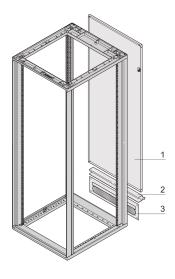
Novastar Rear Panel With Cable ducting for ease of cable management.
