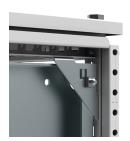
These fixation brackets allow for fitting a full height or partial height mounting plate to one side within the enclosure when more mounting space is needed. The mounting plate will separate bayed enclosures in full, or partially, depending on the height of it.
