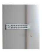
The DIP profile system is a 40 mm wide and 25 mm high profile, which can be mounted on the enclosure depth. It can also be used in combination with CLPF and CLPK profiles. Two rows of holes patterns for cage nut fixing and self-tapping screws are provided. DIP profiles are not compatible with adjustment in depth of the mounting plate.
