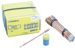
The nVent ERICO Cadweld bootleg bonds are intended to be welded to the web of the rail at the rail profile neutral axis level. To ensure connection integrity, the attachment shall be made using nVent ERICO Cadweld welding material.
