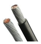
Theft-deterrent composite cables (TDCC) are conductors that function as copper conductors, but appear to be non-copper conductors and are difficult to cut and steal. These conductors are ideal for exposed electrical distribution grounding leads where copper theft may occur. Theft deterrent conductors are difficult to cut with hand tools and the outer steel stranding is magnetic, which further deters thieves looking for copper.
