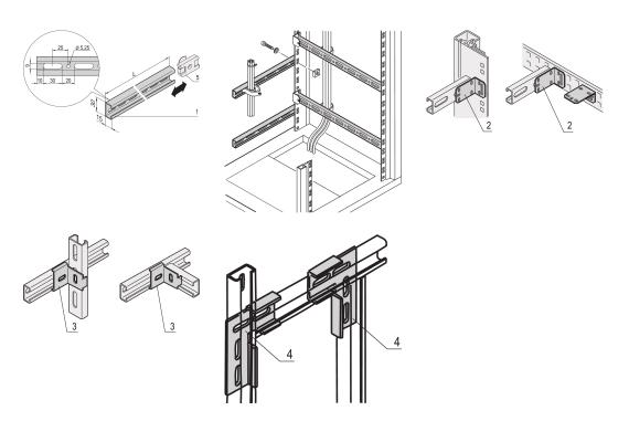
For assembly to the vertical uprights on the right and left hand side of the 19" plane; especially suited for cable eyes.
