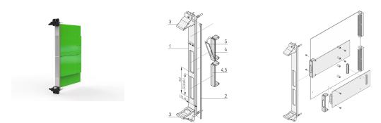
U-shaped front panel with cutout for PMC. Shieldable for textile EMC gasket.
