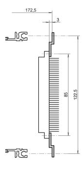
Z-rail for connector in accordance with DIN 41617, 31-pin.
