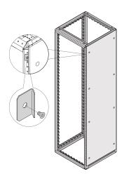
The internal retainer is easily fitted without drilling, and allows the side panel to be removed only from inside. The retainer is only for IP 20 applications.
