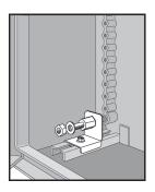
Ultrx Panel Bracket Kit is used with panels and allows panel adjustment from front to rear. Fits all Ultrx enclosure sizes. Mounts on integrally molded body rail. All mounting hardware is included.
