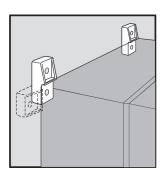
Ultrx Mounting Bracket Kit is field-installable. Type 316 stainless steel mounting hardware included. Four mounting brackets per kit.
