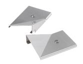
Clean Tray transition covers are used for Transitioning from a sloped to standard cable tray. Available with right- and left-hand slope. Will fit the Splice (order separately) or anywhere on a straight section (transition cover sloped to flat left-hand shown in drawing). The Clean Tray stainless steel system is designed to protect rated cabling in applications that require frequent washdown.
