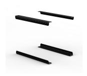
Side crossbar to support 19" uprights in a 800 mm wide cabinet supporting 800 kg static load. The hole pattern allows easy reccessment of the 19" plane in 25 mm increments.
