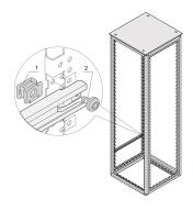
Assembly Kit for mounting Accessories directly on the Varistar CP Frame from the outside or inside.
