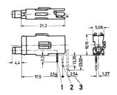
Test sockets for mounting plane 1 and 2, short and long type.
