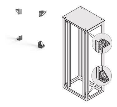
Varistar Adapter Bracket for reduced Width for the assembly of 2 panel/slide mounts. It comes in combination with the assembly of depth members, recessed of shortened 19" panel/slide mounts.
