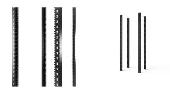
Slide mout with adjustable increments. Assembly in 600 mm wide cabinets directly on the frame. At 800 mm width adapter bracket for reduced width is necessary, for partial-height mounting depth members are necessary.
