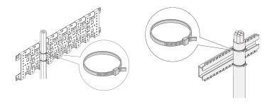
Assembling materials kit for cable routing.
