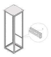
Varistar horizontal cable support rail in the cabinet width. Mounted directly at the frame.
