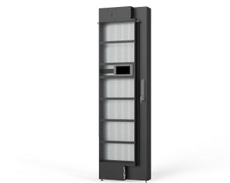
The new rear door cooling units from nVent are offered in a range of standard sizes for use with 42U, 47U, in both 600mm and 800mm widths (other sizes available on request). The coolers themselves are 250mm deep, with a dry weight of 140Kg. One of the features of rear door coolers is they are compact and do not require any additional floor space or ceiling headroom – in fact, their use can free up white space as CRAH units and other room cooling equipment may be eliminated from the data centre.
