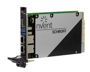
The nVent SCHROFF PXIe embedded controller is the most compact and powerful 3 U/4 HP embedded controller for PXI Express and CPClexp platforms. With its comprehensive and future-proof interface and compute power capabilities, it is ideally suitable for test and measurement applications. The controller is driven by a 11th generation Intel® Xeon® processor, combined with up to 64 GB DDR4 memory and supports high bandwidth applications with PCIe Gen4 and 10GBASE-T interconnectivity.
