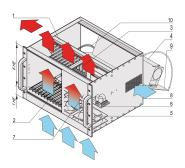
VME system for 12 VME boards 6 U, 160 mm. The power for the system is supplied by an open frame power supply. A fan control module monitors the fans, the temperature and voltage.
