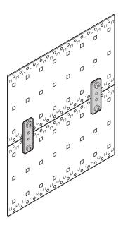
The brackets are used to connect the fan units to the side panels of a subrack.
