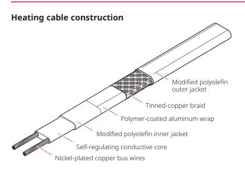
Raychem HWAT self-regulating heating cables are installed on hot water supply pipes underneath standard pipe insulation. The heating cable adjusts its power output to compensate for variations in water temperature and ambient temperature. The heating cable replaces supply-pipe heat losses at the point where the heat loss occurs, thereby providing continuous, energy-efficient, hot water temperature maintenance and eliminating the need for a recirculation system.
