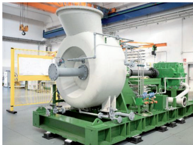
Figure 4 Exergy's Radial Outflow Turbine
