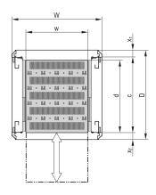
Varistar 19" Shelf, Stationary with 30 KG load capacity, perforated for ease of assembly.
