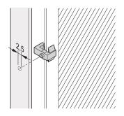
Fixing clip for PCB assembly to front panel with extractor handle keyform 1.
