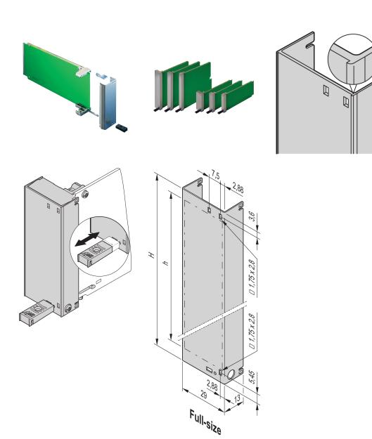
AdvancedMC Front Panel including EMC gasket for AMC.0 Rev. 2.0 Modules.
