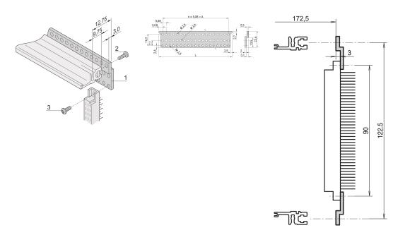
Z-rail for connector in accordance with EN 60603-2 (DIN 41612).
