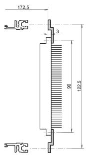
Z-rail for connector in accordance with EN 60603-2 (DIN 41612).
