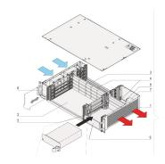
2 U CompactPCI System with horizontal Card Cage for four 6 U Boards, four RTM Boards and one CompactPCI 3 U Pluggable Power Supply. Option to assemble a second pluggable Power Supply.
