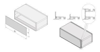
The EMC front panel can be inserted in special horizontal rails with an elevation. No screws are needed for the fixing. The design enable a users to use a front foil.
