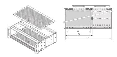
A cover plate is used for electromagnetic shielding or as mechanical protection.
