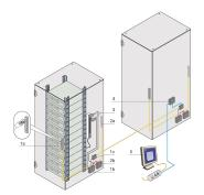
Electronic handle with transponder card reader. The handle opens when recieving a signal from an authorized tansponder card.
