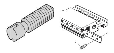
For fixing the threaded insert in the horizontal rail.
