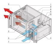
VME system for 8 horizontally mounted VME boards 6 U, 160 mm. The power for the system is supplied by an open frame power supply. A fan control module monitors the fans, the temperature and voltage.
