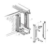
Connector coding is used to provide security against incorrect insertion.
