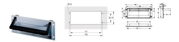
Folding handles can be used instead of the pre-mounted handles shells.
