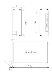
Pluggable 19" Power Supply with P47 connector, for CompactPCI applications.
