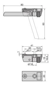
The tip-up feet from aluminum die cast material enable mounting on the bottom plate of a case. Available with or without tip-up function. Color RAL 9006 White Aluminum.
