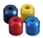
The nVent LENTON Grommet is used in conjunction with the nVent LENTON Bolted Form Mount and nVent LENTON Toggle Form Mount. These Grommets are used to secure nVent LENTON Interlok Grout-Fill Coupler variants in repeatable locations in the formwork. Once a Grout-Fill Coupler is placed over a Grommet, the Form Mount bolt is tightened, which expands the outside diameter of the Grommet, thus holding the Grout-Fill Coupler in place.
