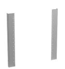
Rack mounting angles are designed for standard 24-in. (610-mm) wide one-door, Wall-Mount Type 4 and 12 enclosures. A pair of pre-cut rack mounting angles are available for mounting 19-in. (483-mm) rack-mounted equipment. To install, drill small holes in the sides of the enclosure and bolt angles in place.
