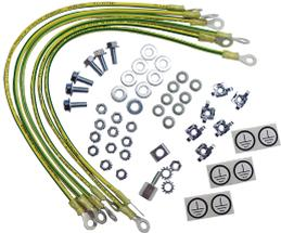
The Grounding Kit allows a ProLine or ProLine G2 enclosure to be grounded to VDE specifications. Includes six 12-gauge wires 411 mm (16.19) long with ring terminations and M6 mounting hardware.
