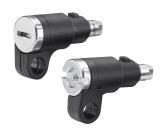
Padlock Inserts fit into standard quarter-turn latches. Made of black composite material (PBT) with zinc insert and replace the standard 3-mm double-bit or slotted screwdriver insert when padlocking security is required.
