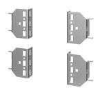
Frame-Reducing Brackets mount directly to 700- or 800-mm wide ProLine frames or to grid straps. Converts wider frames to 600-mm wide, allowing 19-in. rack angles to fit, or to 700-mm wide, allowing 23-in. rack angles to fit. Can be used to left- or right-justify the rack-mounted equipment. Furnished in sets of four. Mounting hardware is included.
