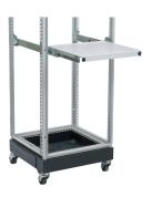
Frame Pull-Out Shelf allows easy access to shelf-mounted devices. The shelf has 12 gauge steel supports. The shelf mounts to the front and rear frame uprights. The load rating is 110 lb. (50 kg).
