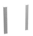
Rack mounting angles are designed for standard 24-in. (610-mm) wide one-door, Wall-Mount Type 4 and 12 enclosures. A pair of pre-cut rack mounting angles are available for mounting 19-in. (483-mm) rack-mounted equipment. To install, drill small holes in the sides of the enclosure and bolt angles in place.
