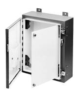
Swing-Out Panel Kits allow mounting standard junction box and NEMA style panels (purchase separately) near the front of the enclosure for easy access to or reading of gauges, switches, pilot lights and other components. Kit consist of heavy-gauge brackets and hinges which are easily installed by drilling small holes in the sides of the enclosure and bolting the brackets in place.
